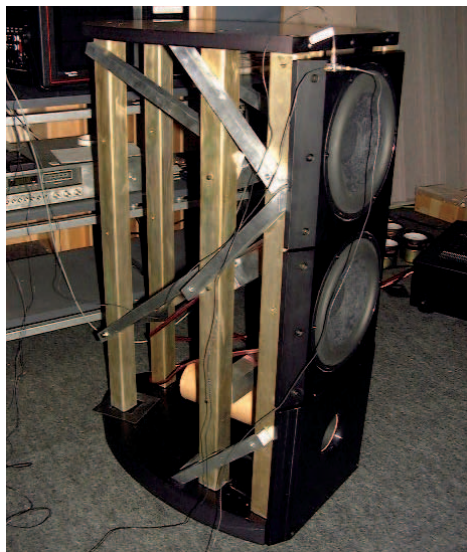
Kaku built and tested this laboratory prototype, which features extensive metal cross-bracing.
