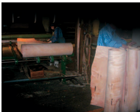
Peeling the logs to create a continuous sheet of maple laminate.
